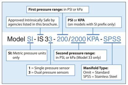
This manual applies to all models in the current 30 Series product line. To determine the specifications for your model, use this table to decode the model number.
