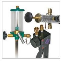
Crystal offers three different handpump options. All provide a portable pressure source for the calibration of 30 Series calibrators, as well as other high pressure gauges, recorders, switches and transmitters. A built-in variable volume control makes it easy to set precise pressure with the turn of a dial. Additionally, the CylinderPump and ComboPump can serve as both a pressure and vacuum source.
